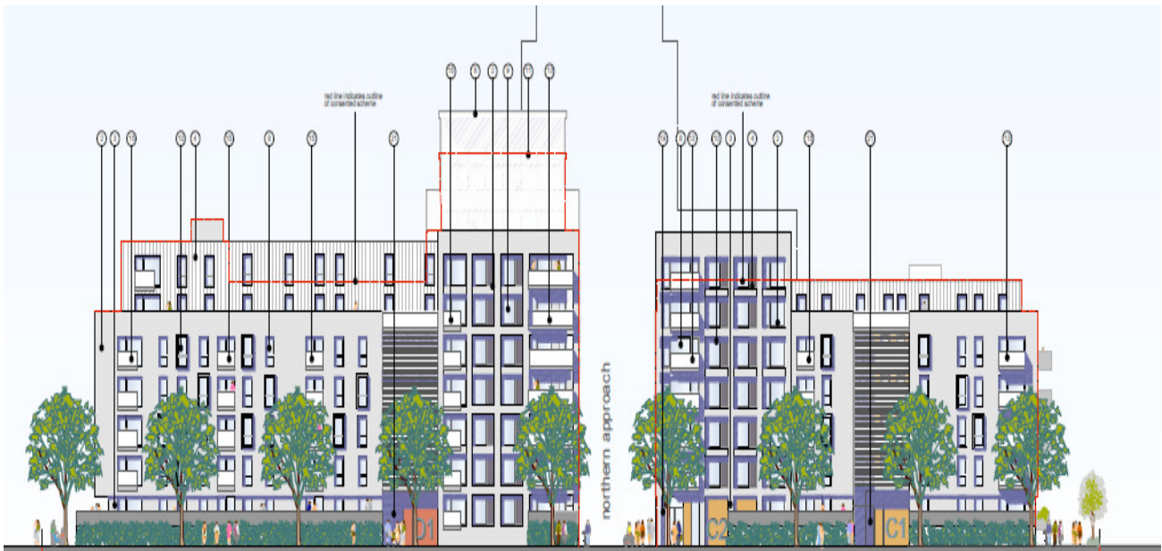
Elevation 1: Showing the Bartlett Park (Lindfield Street elevation) as proposed. The red line outlines the height of the consented scheme.
